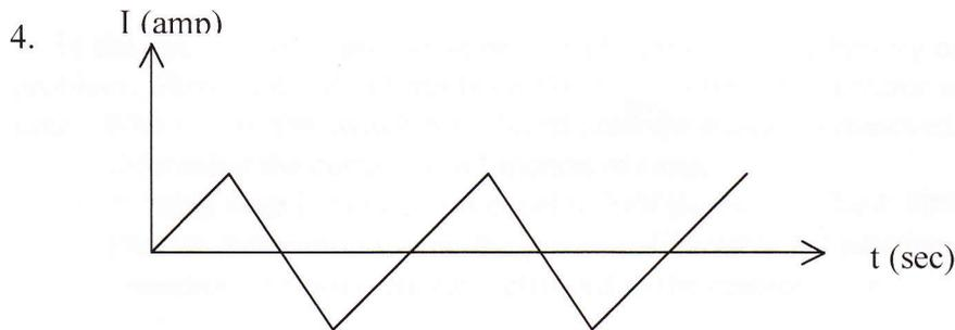
The graph above represents the current passing through an inductor. Draw a graph representing the voltage across the inductor.
