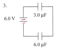
a. In the circuit above, determine the total capacitance. Find how much charge is on each capacitor, and find the potential difference across each capacitor.
